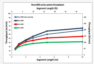
Note : the 840i and 860i have the identical throughputs for both commercial wide spacing and military close coded spacings, whereas the 880i performs at a slightly higher speed for commercial spacings
