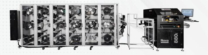
Nova wire markers comply with all key OEM aerospace specifications and international standards, including SAE AS 5649 and ASD EN4650, "Wire and cable marking process, UV laser".
